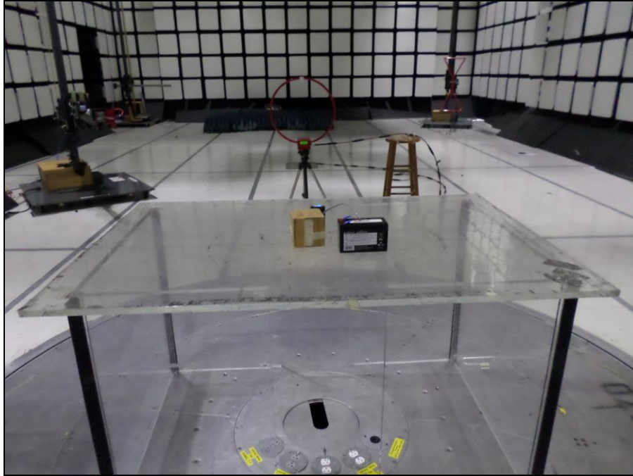
Photograph 7. Spurious Emissions, Outside the Band 13.110 - 14.010 MHz, 9 kHz – 30 MHz, Rear View
