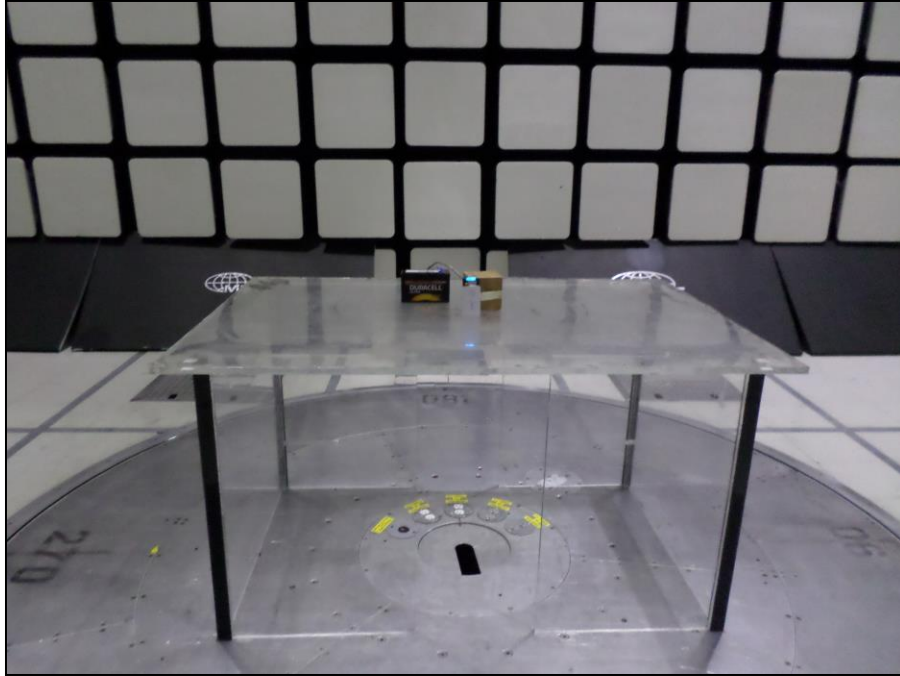
Photograph 5. Spurious Emissions, Outside the Band 13.110 - 14.010 MHz, 9 kHz – 135.6 MHz, Front View
