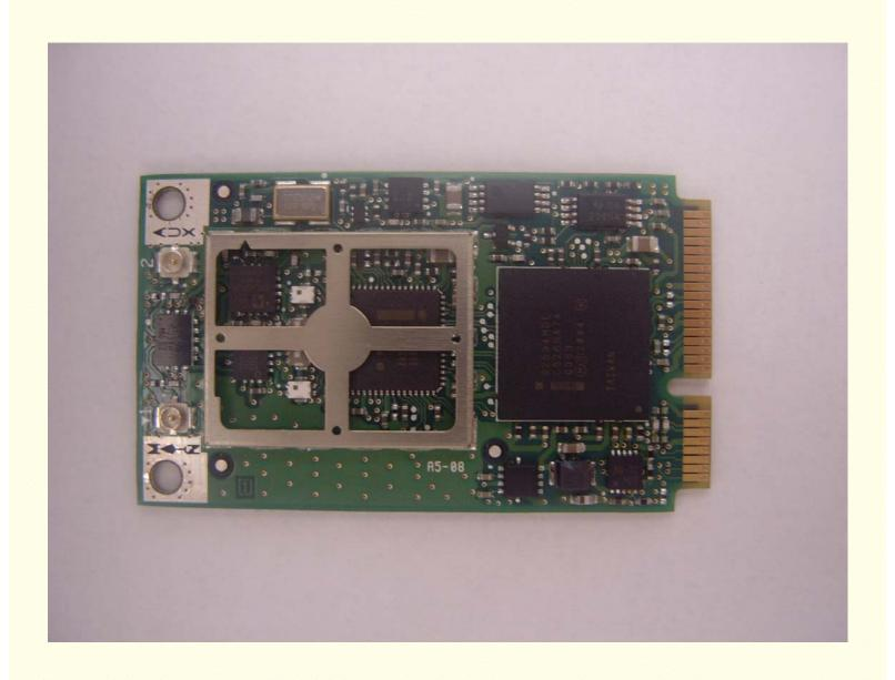
Top View "Shielding removed"
