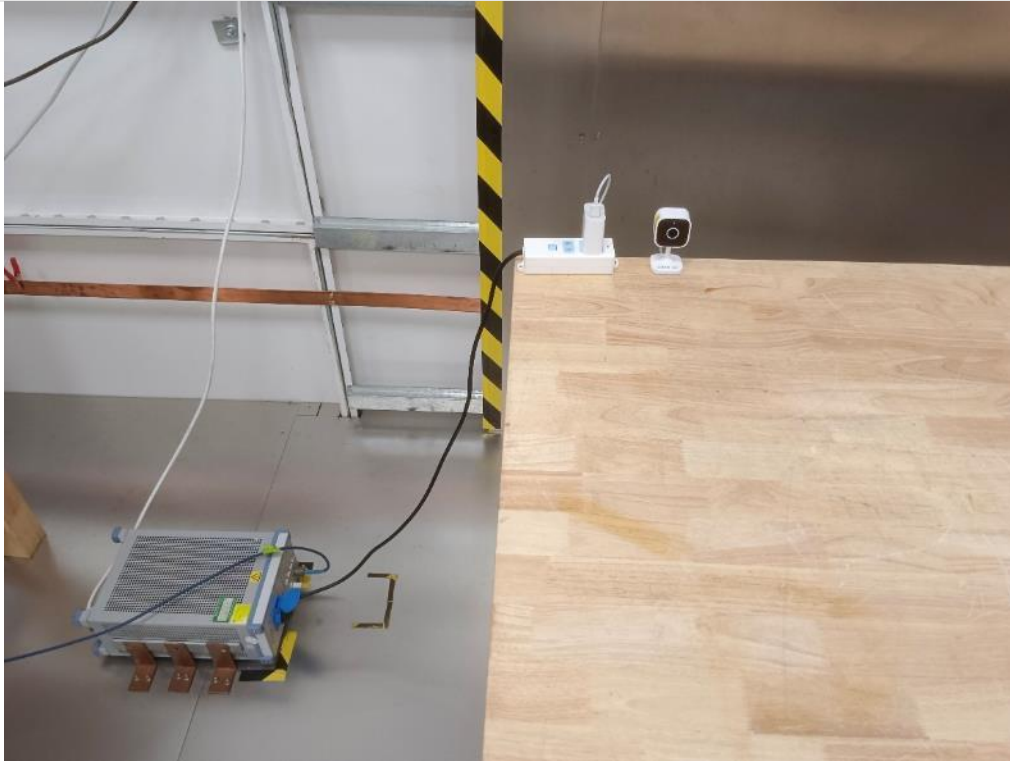
AC Power Line Conducted Emission
