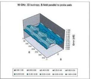
Probe isotropy for E<sub>tot</sub>: probe rotated  $\phi$  = 0° to 360°, tilted from field propagation direction  $\overline{k}$  Parallel to the field propagation ( $\psi$  =0° - 90°) at 30 GHz: deviation within  $\pm$  0.36 dB Parallel to the field propagation ( $\psi$  =0° - 90°) at 90 GHz: deviation within  $\pm$  0.26 dB
