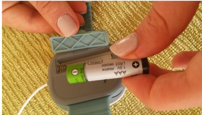
**Figure 5 – Battery insertion**
