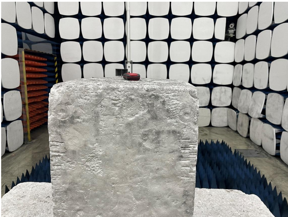
FCC Radiated Emission Test Setup-above 1GHz
