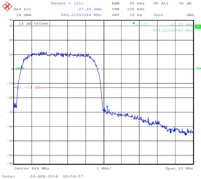
**Cellular Band, Left Band Edge for HSUPA (BPSK) Mode**
