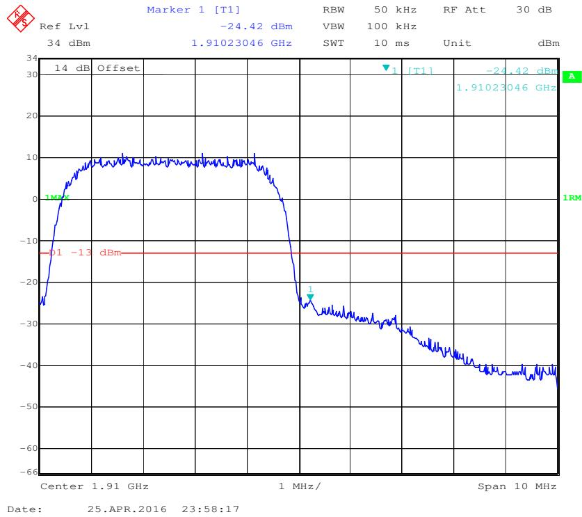
**PCS Band, Left Band Edge for HSDPA (16QAM) Mode**
