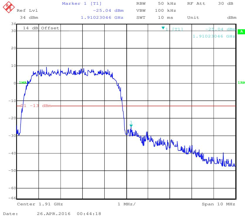
**PCS Band, Left Band Edge for HSUPA (BPSK) Mode**
