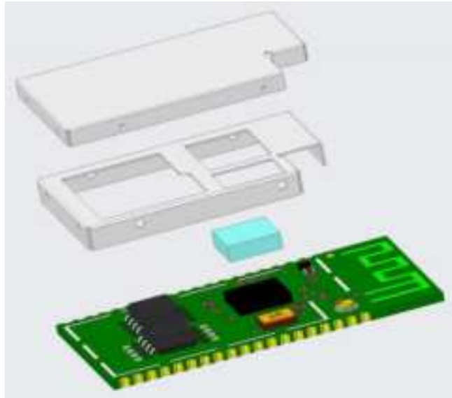
Figure 2.1 Schematic diagram of module structure
