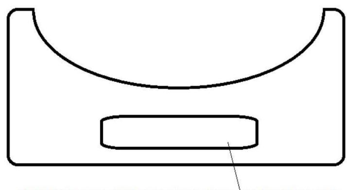
The Label is located inside the compartment of connector slots, which must be seen when the AC power line plug into the device before turnning it on.
