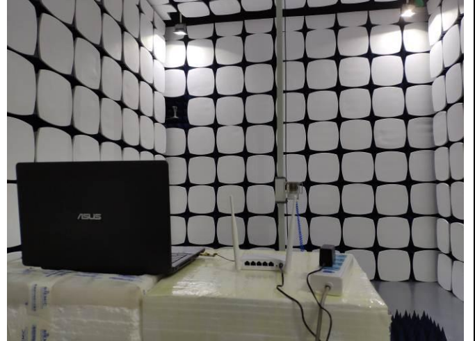
Radiated Spurious Emissions Test Setup Above 1GHz
