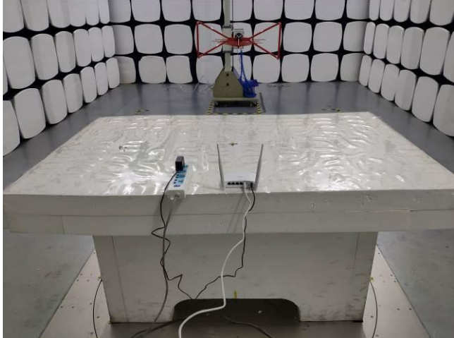
Radiated Spurious Emissions Test Setup Below 1GHz
