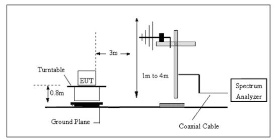
(C) Radiated Emission Test-Up Frequency Above 1GHz
