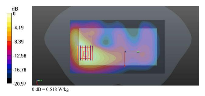
Communication System: UID 0, WIFI (0); Frequency: 2437 MHz; Duty Cycle: 1:1.026
