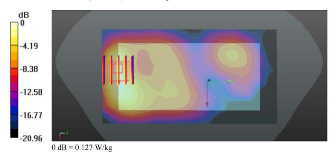
Communication System: UID 0, LTE (0); Frequency: 2560 MHz; Duty Cycle: 1:1
