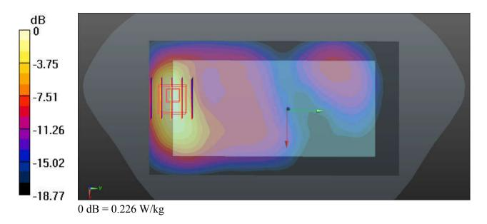
Communication System: UID 0, LTE (0); Frequency: 836.5 MHz; Duty Cycle: 1:1
