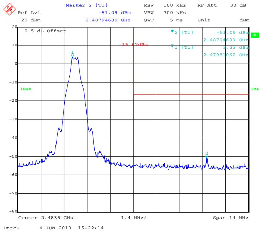
*EDR Mode ( $\pi/4$ -DQPSK):***Band Edge, Left Side**
