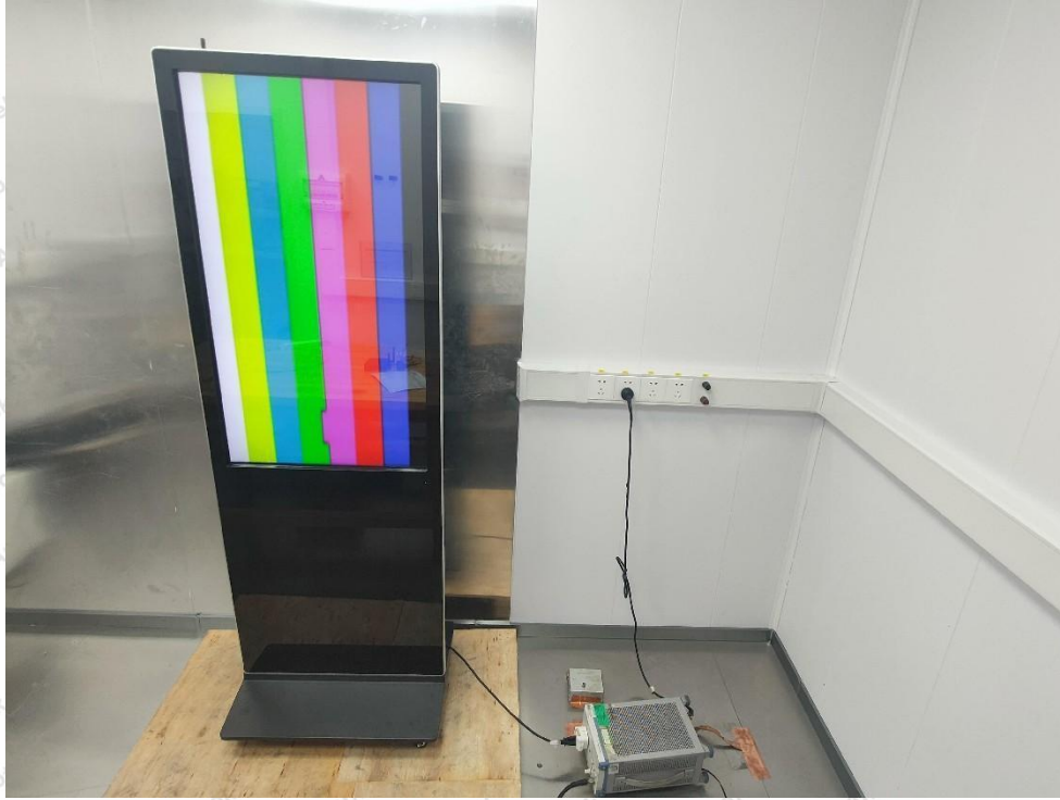
Photo of Radiation Emission Test (below 1GHz)
