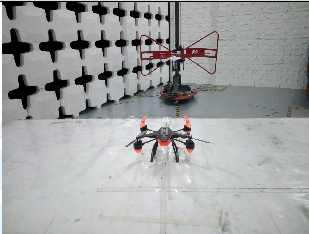
Radiated emission Test Setup (30 MHz~1 GHz)
