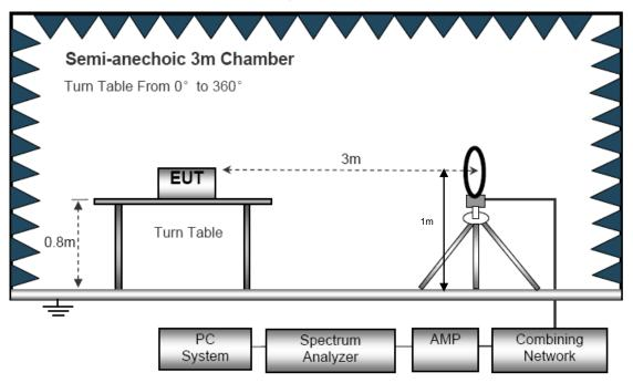
(B) Radiated Emission Test-Up Frequency 30MHz~1GHz
