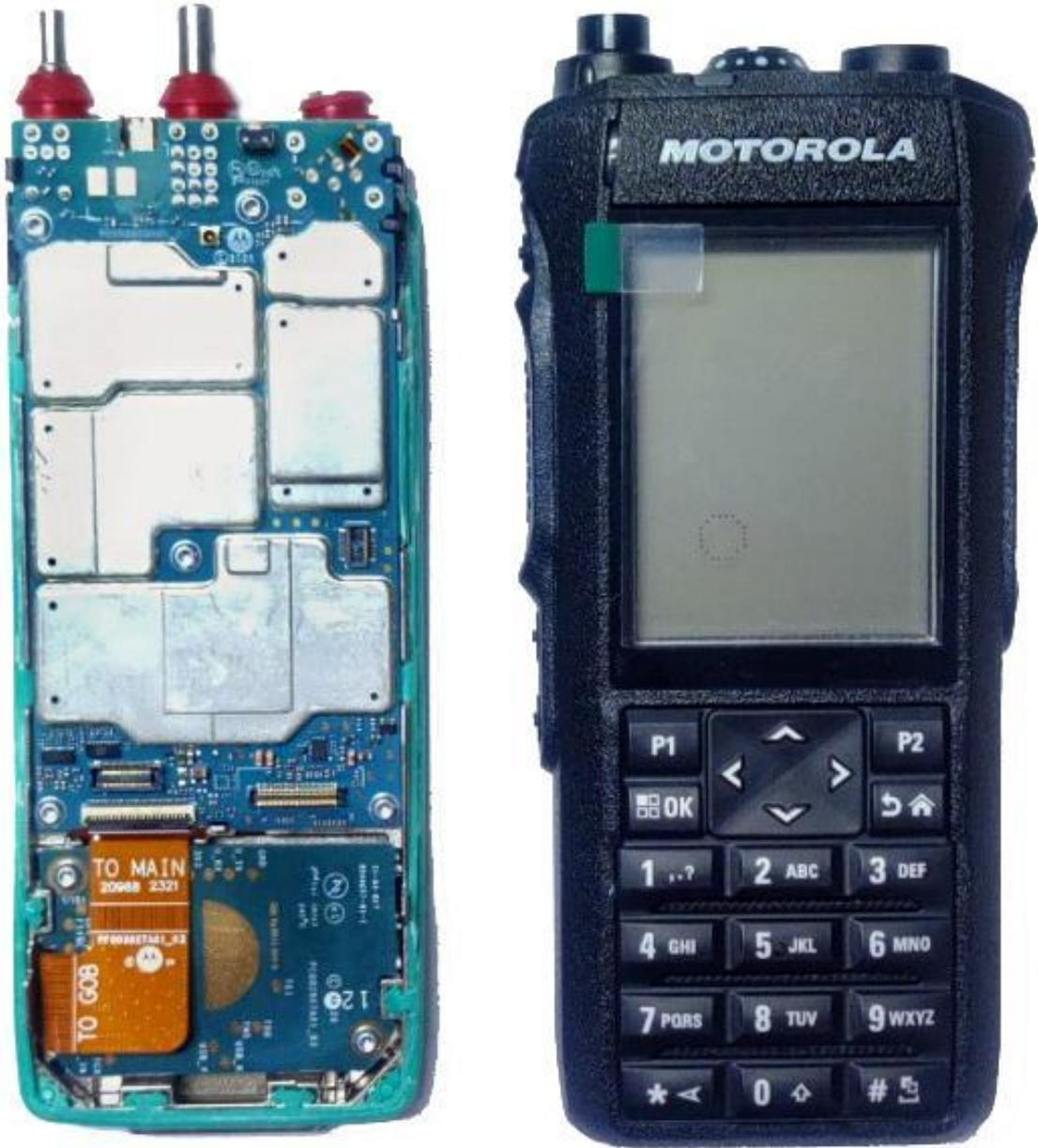
RF board with chassis and housing (front side) of FKP TIA/non-TIA Model
