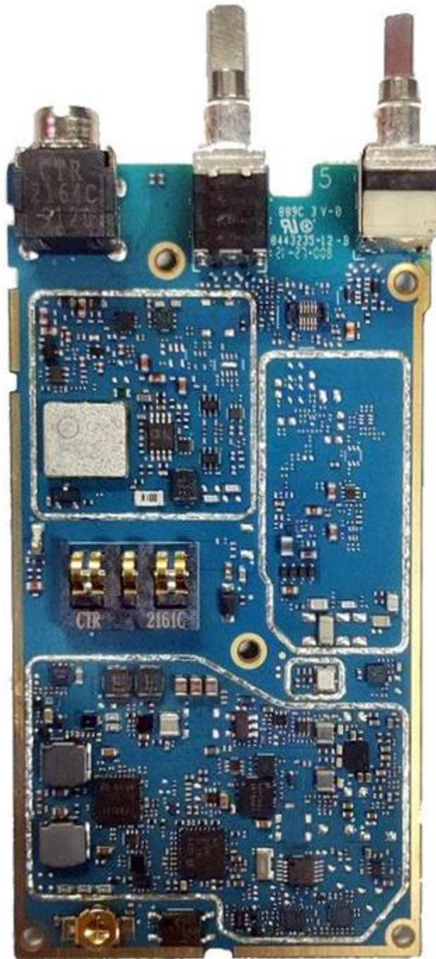
RF board without Shields (Bottom) of FKP non-TIA Model
