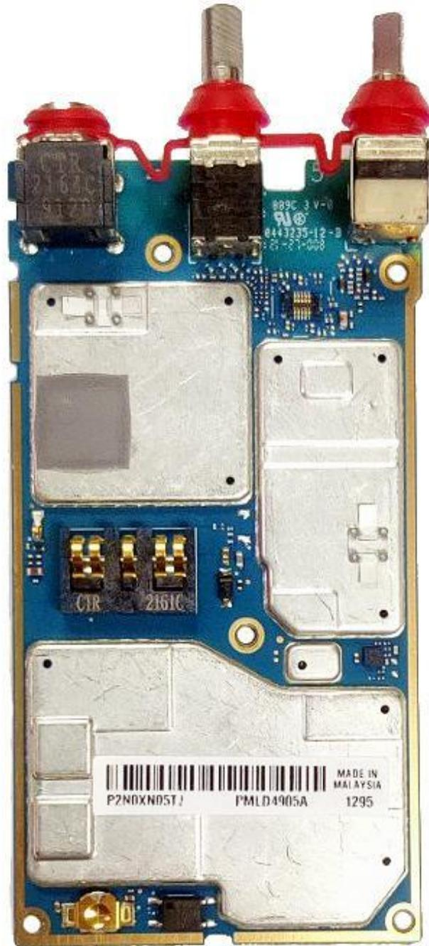
RF board with Shields (Bottom) of FKP TIA/non-TIA Model
