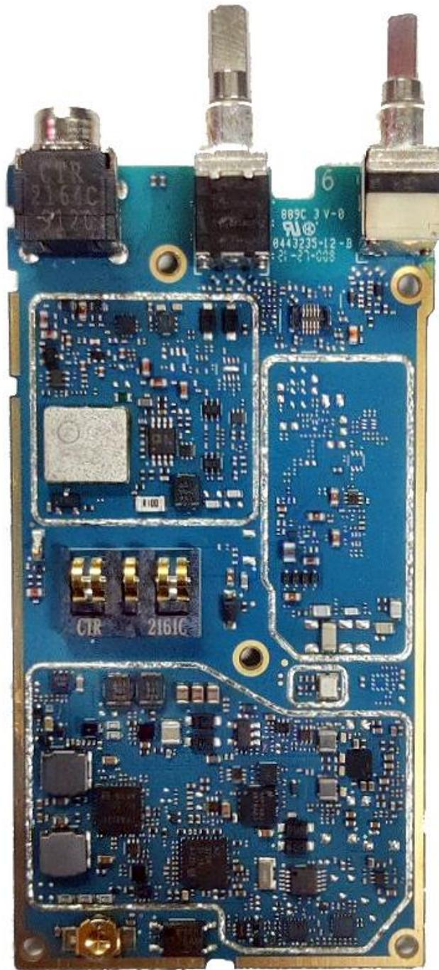
RF board without Shields (Bottom) of NKP TIA Model
