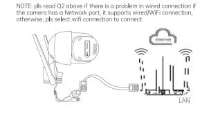
Connect to the router LAN port through a network cable
