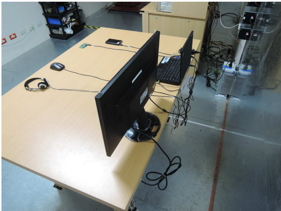
Photograph 5: Set-up for for Mains Conducted testing Back
