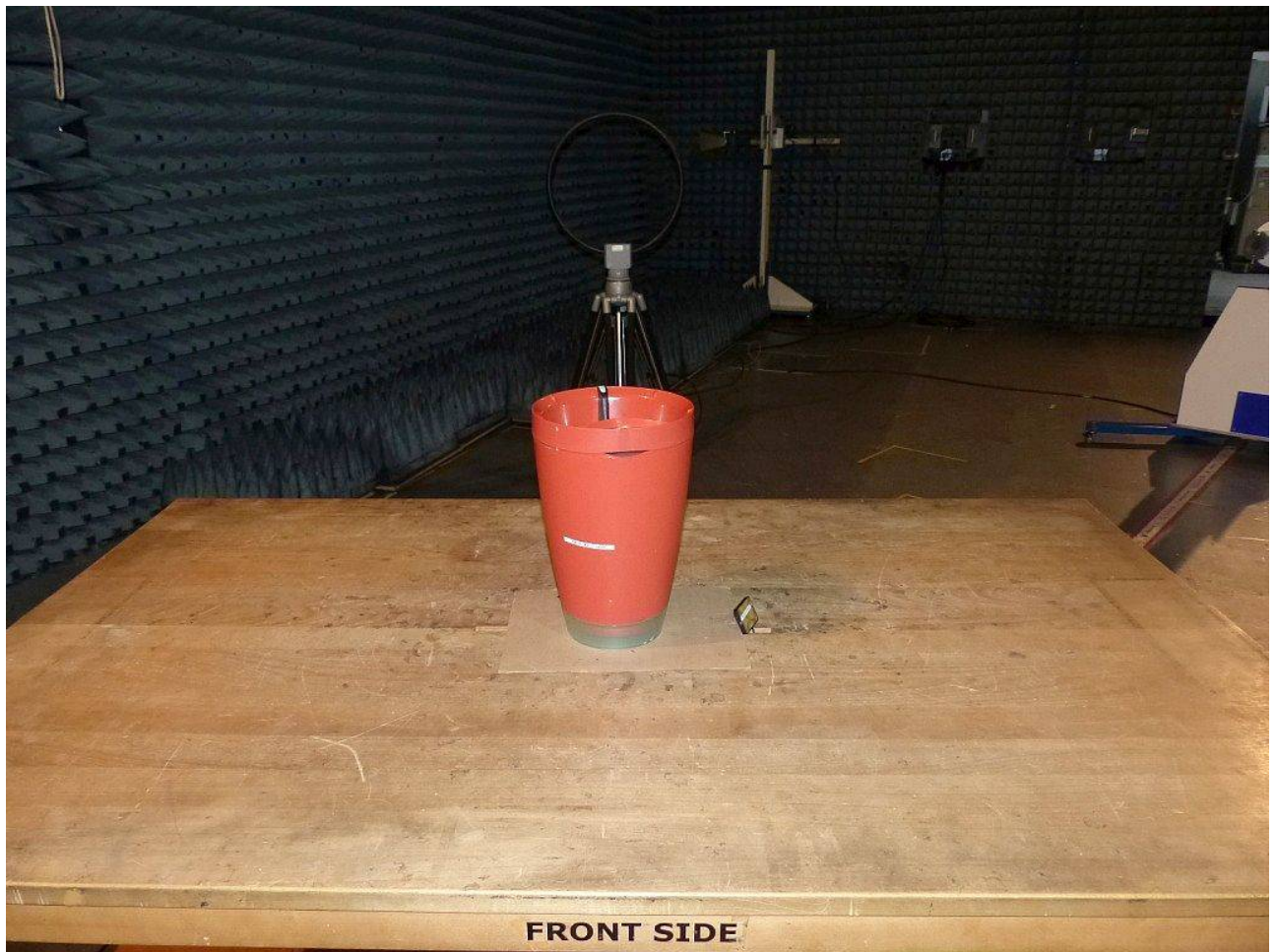
Photo 1: Test setup for radiated measurements (Enclosure, below 30 MHz, intentional radiator §15, ANSI C63.10)
