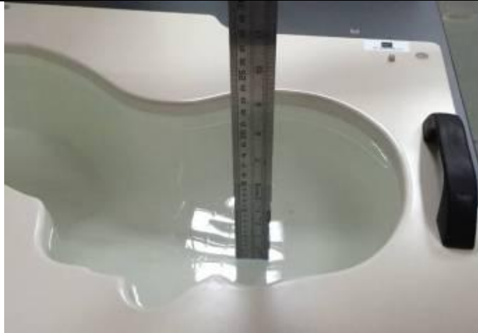
Head Position with 5000MHz liquid depth (15.3cm)
