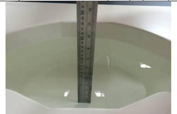
Body Position with 5000MHz liquid depth (15.2cm)
