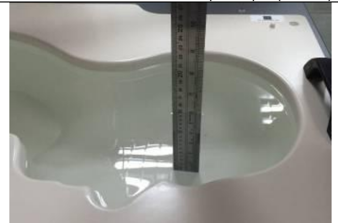
Head Position with 5000MHz liquid depth (15.3cm)
