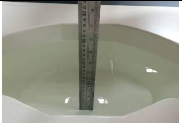
Body Position with 5000MHz liquid depth (15.2cm)
