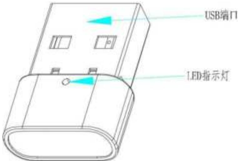
1, power on: in the shutdown state, insert the USB port into the computer device and power on the "product", and then power on the computer
