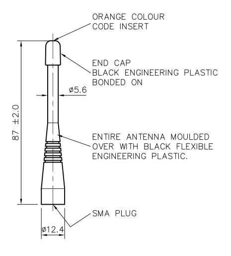
SPR-03072 No. TITLE 300-00498 1/4 WAVE WHIP XW BAND 806-870 MHz. MATERIAL FINISH DRAWN DO.CHECK B.L. SCALE 1:1 DIMENSIONS IN mm TOLERANCES UNLESS OTHERWISE STATED O DEC. PLACE ±0.5 2 DEC. PLACES ±0.1 1 DEC. PLACE ±0.2 ANGULAR DO NOT  $\bigcirc$ PROJECTION SCALE C/NOTE ISSUE DATE 30.04.08 01019
