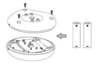
Note: After replacing the battery, you need to align the positioning points of the upper and lower shells to close the cover and then screw the device closed.
