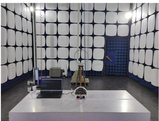
3. Radiated emission (9KHz-30MHz)
