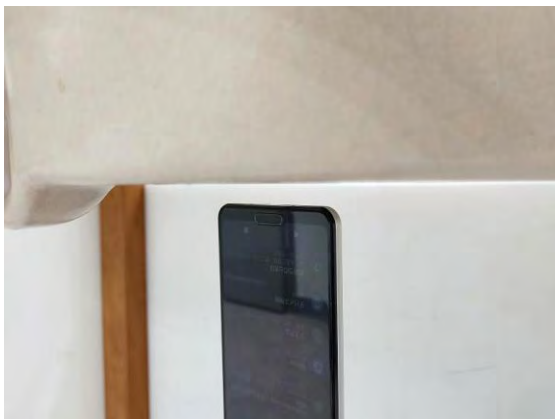
Fig.11 EUT Bottom side to flat phantom
