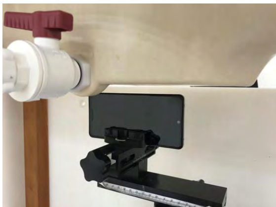
Fig.13 EUT Left side to flat phantom
