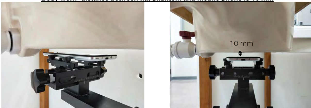
Fig.7 EUT Front side to flat phantom
