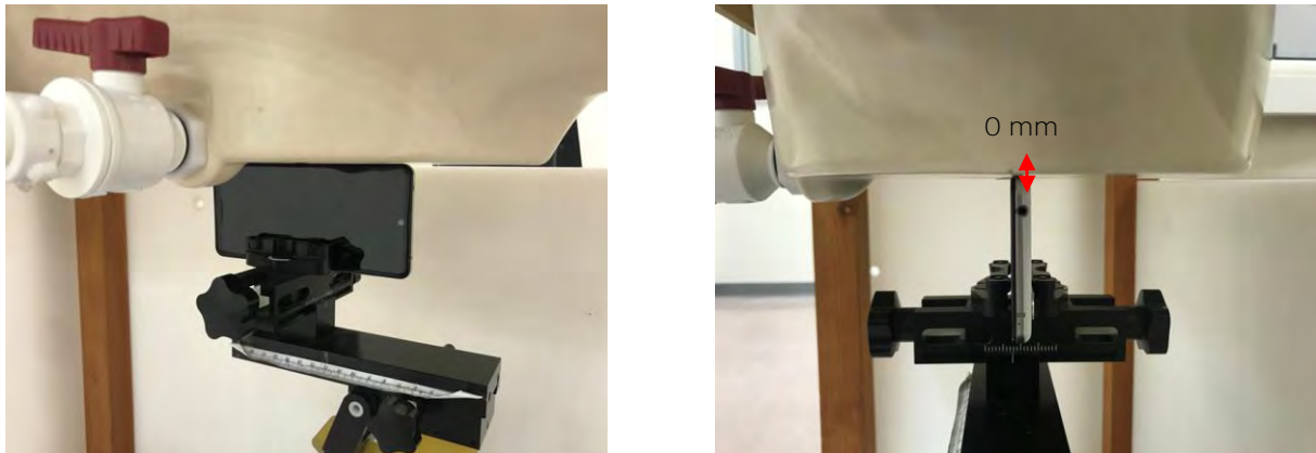
Fig.19 EUT Left side to flat phantom
