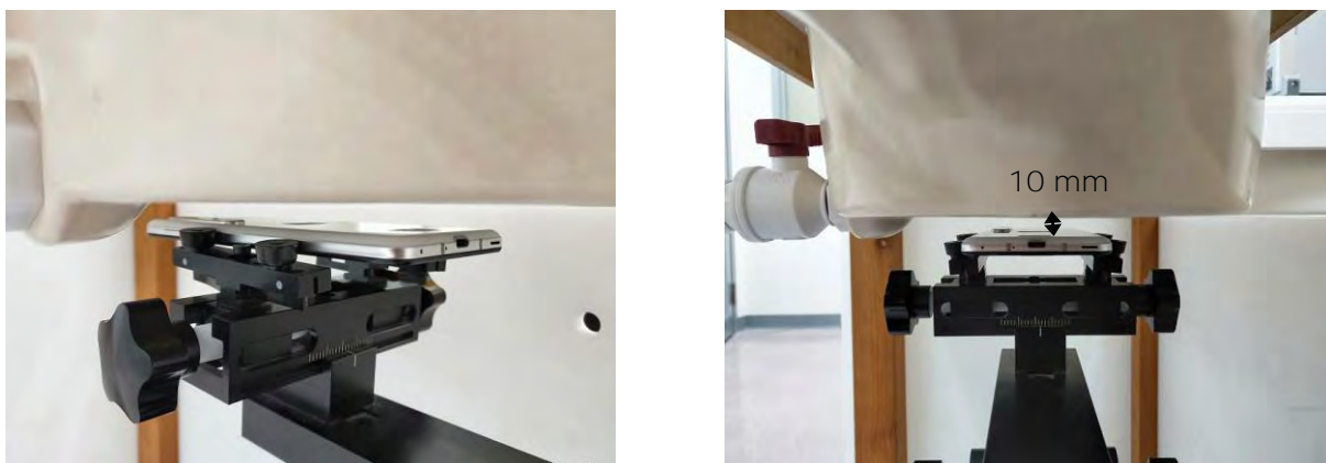
Fig.8 EUT Back side to flat phantom
