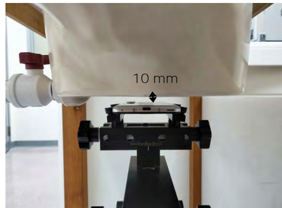
Fig.10 EUT Back side to flat phantom
