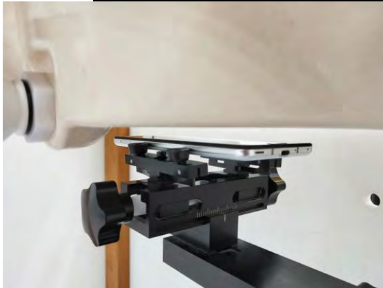
Fig.9 EUT Front side to flat phantom
