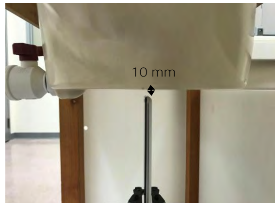
Fig.11 EUT Bottom side to flat phantom
