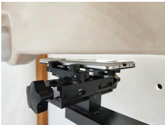
Fig.10 EUT Back side to flat phantom
