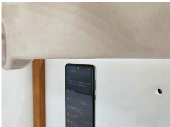
Fig.14 EUT Top side to flat phantom
