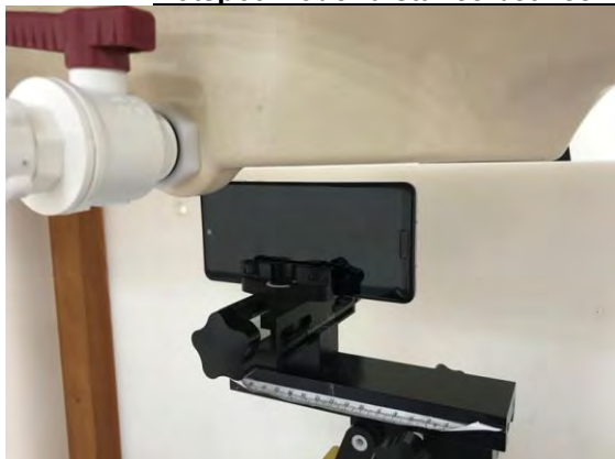
Fig.12 EUT Right side to flat phantom
