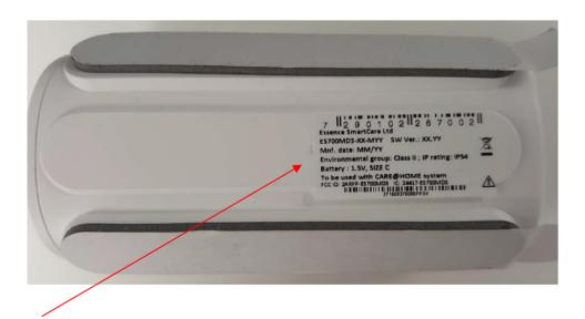
Label with **FCC ID: 2ARFP-ES700MDS and IC: 24417-ES700MDS** will be located here. The statement according to FCC part 15 §15.19(a)(3) is placed in User Manual, page 4 (Application exhibit User\_manual\_37527).
