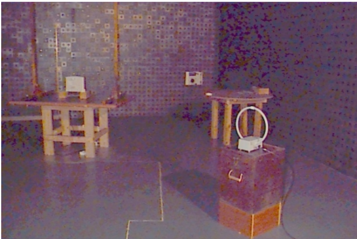
Photograph No. 4.8.1 Radiated emission measurement test setup
