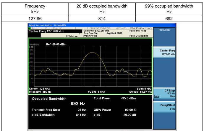
**Note:** Because the measured signal is CW-like, adjusting the RBW per C63.10 would not be practical since measurement bandwidth will always follow the RBW. The RBW is set to 300 Hz to perform the occupied bandwidth test.
