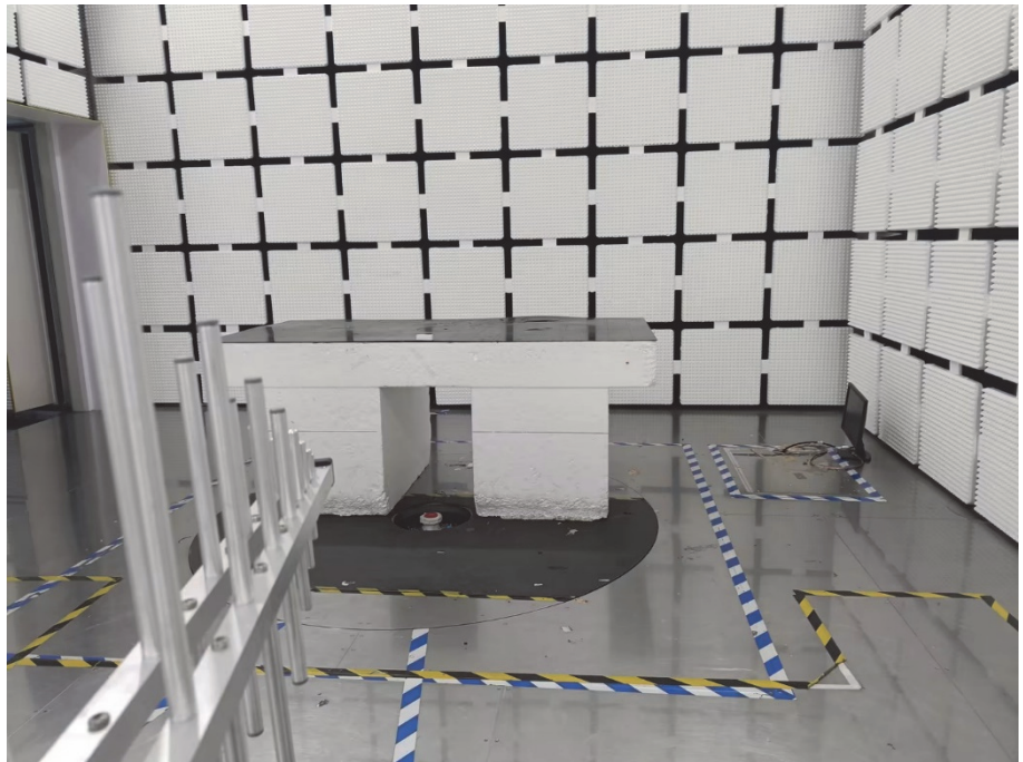
Radiation Emission Test Setup (30MHz to 1GHz)
