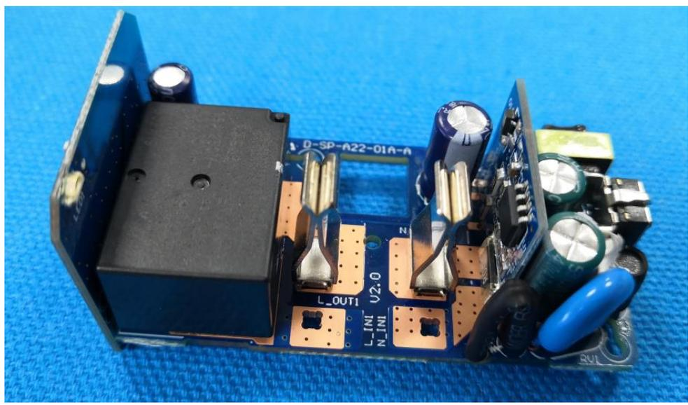
AZ9481 Relay , without power analyzer chip
