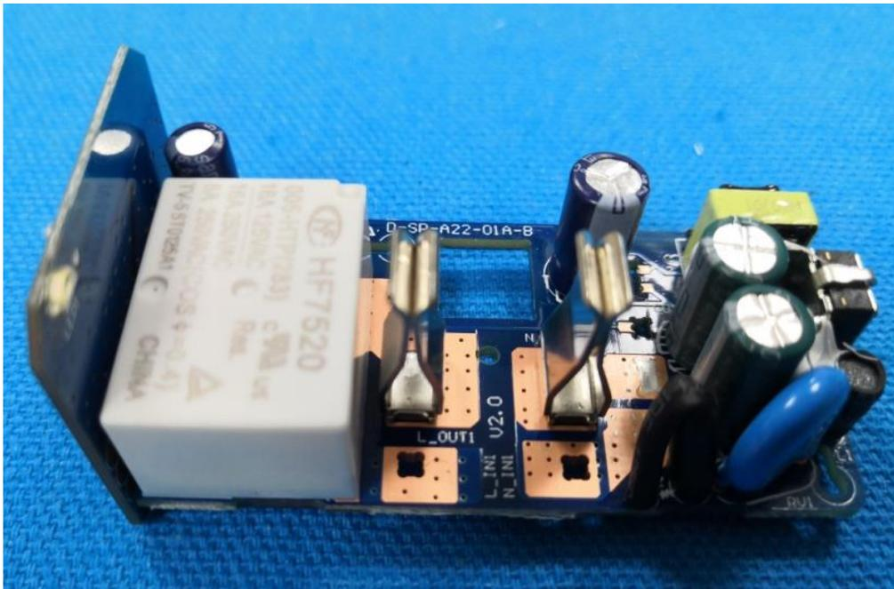
AZ9481 Relay , with power analyzer chip
