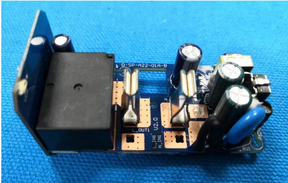
Detail View of EUT-1(with power analyzer chip)
