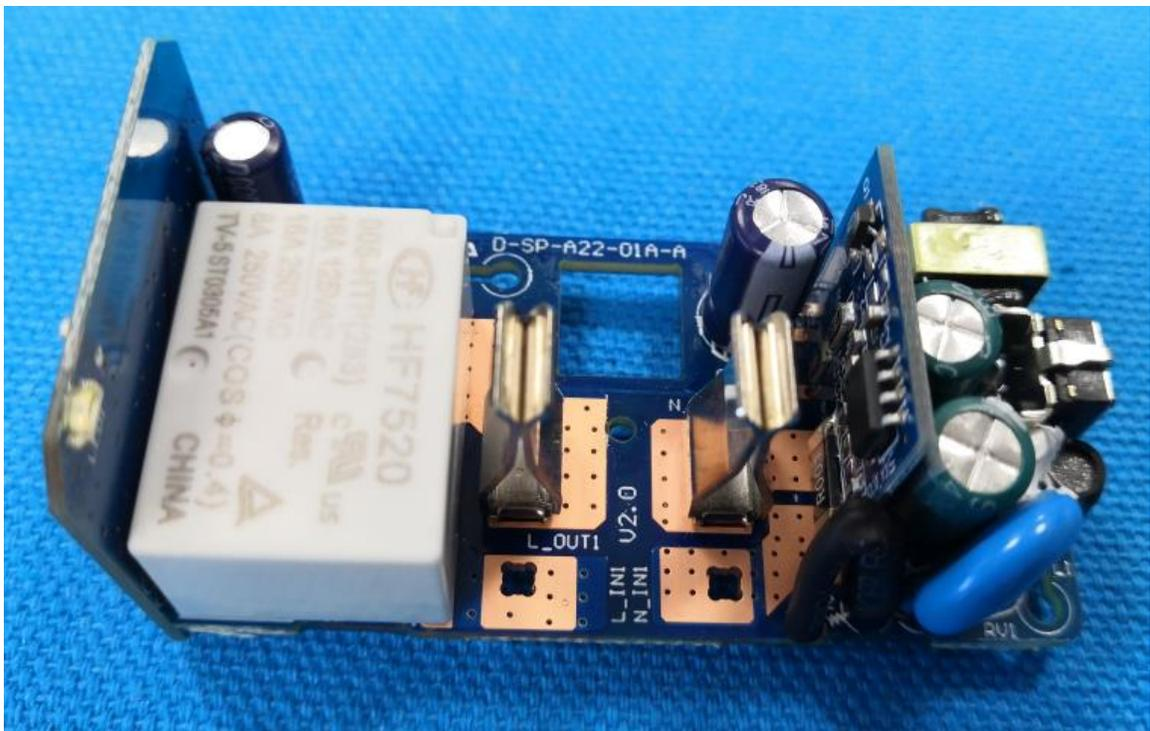
HF7520 Relay , without power analyzer chip
