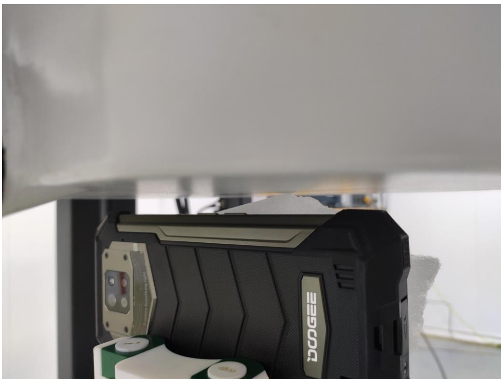
10mm body-worn Left Side Setup Photo (hotspot)
