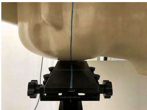
Fig.4 Right Head Section / Ear-Tilt Position(15°)
