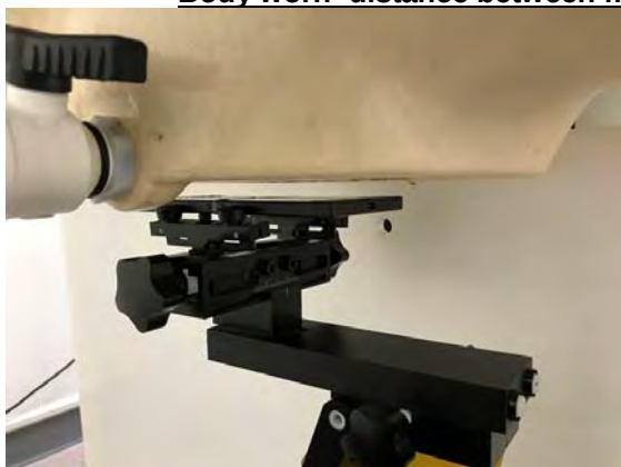
Fig.7 EUT Front side to flat phantom
