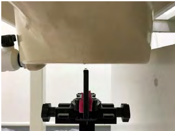
Fig.13 EUT Left side to flat phantom
