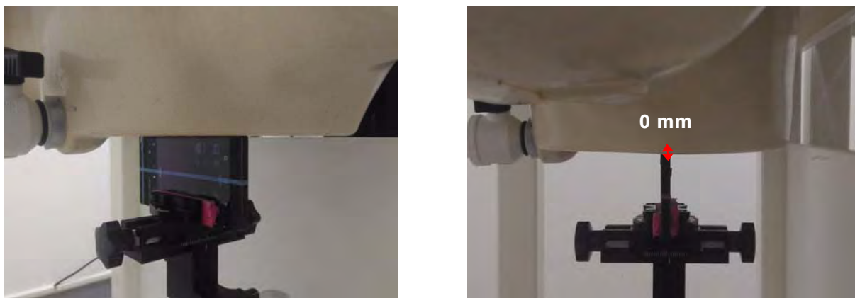
Fig.19 EUT Right side to flat phantom
