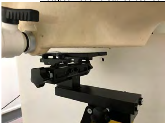
Fig.9 EUT Front side to flat phantom
