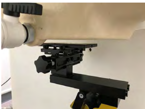
Fig.10 EUT Back side to flat phantom
