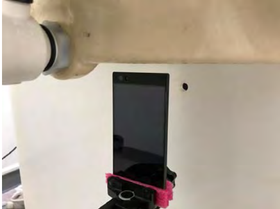
Fig.12 EUT Top side to flat phantom
