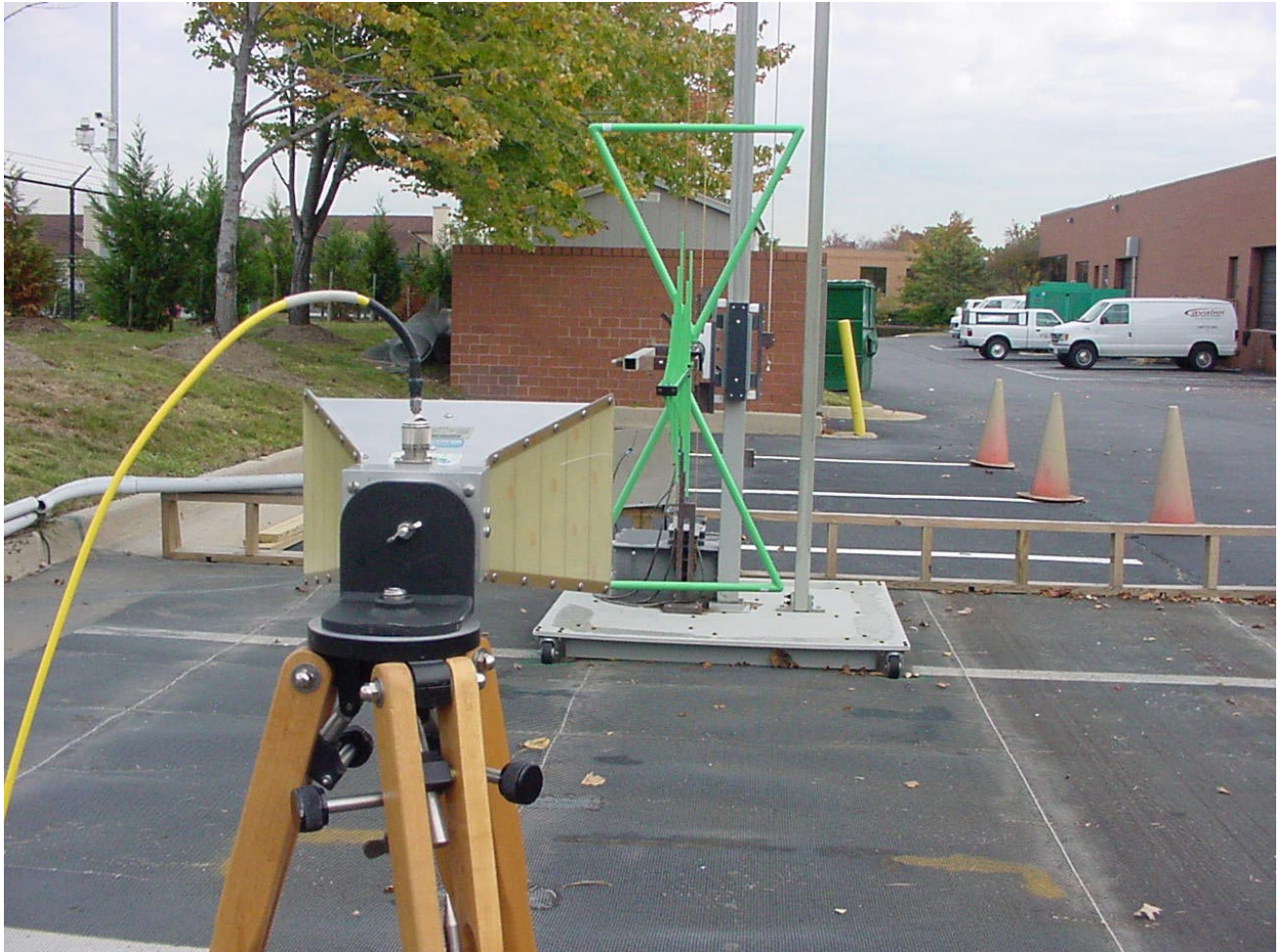
PHOTOGRAPH 5: SUBSTITUTION HORN ANTENNA USED FOR FREQUENCIES (1 GHZ-18 GHZ)
