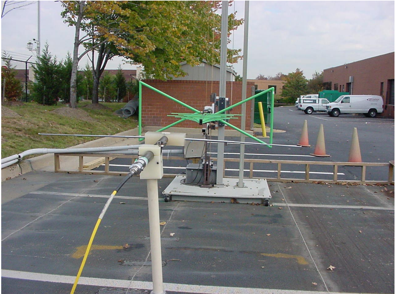
PHOTOGRAPH 4: SUBSTITUTION DIPOLE ANTENNA USED FOR FREQUENCIES (30 MHZ – 1 GHZ)
