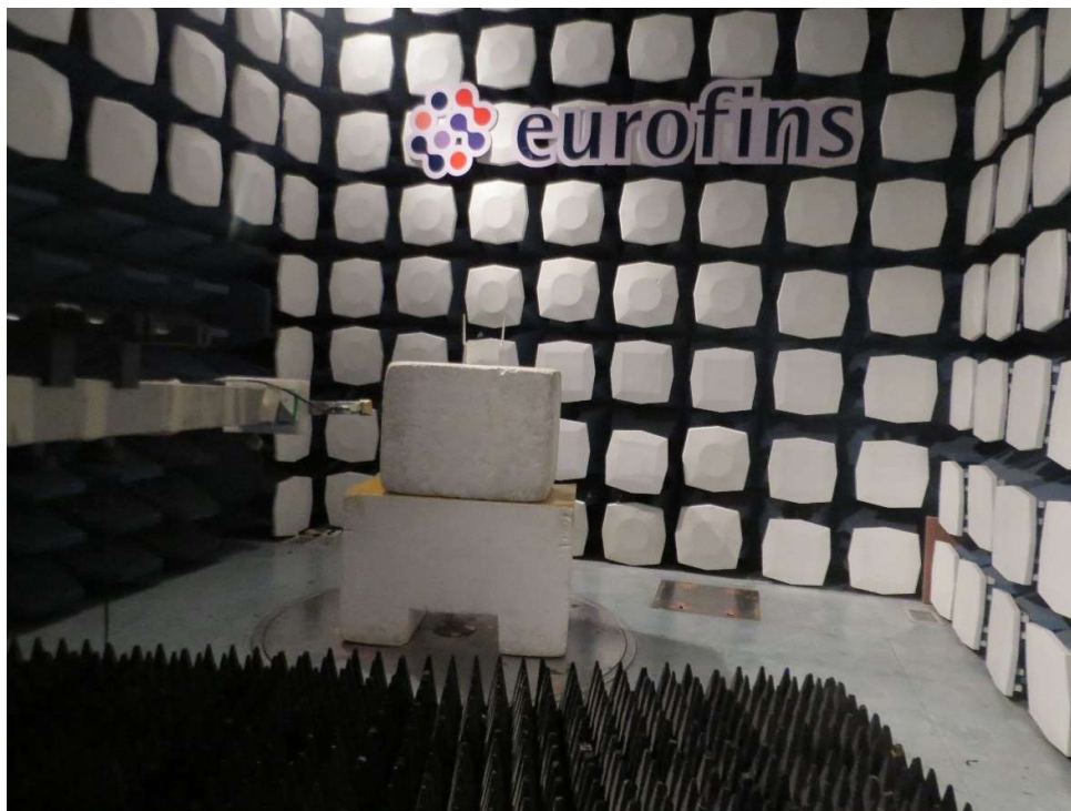
Picture 1 Radiated Emission Test Setup
