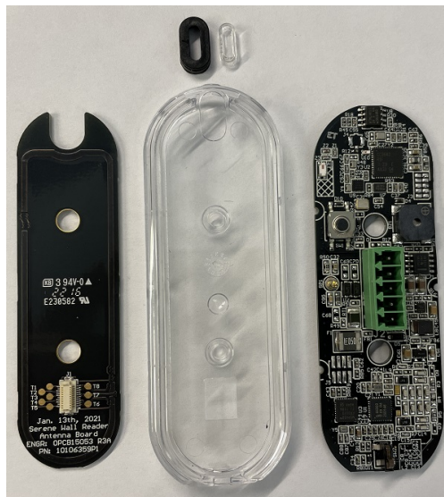
disassembled (potting absent)
