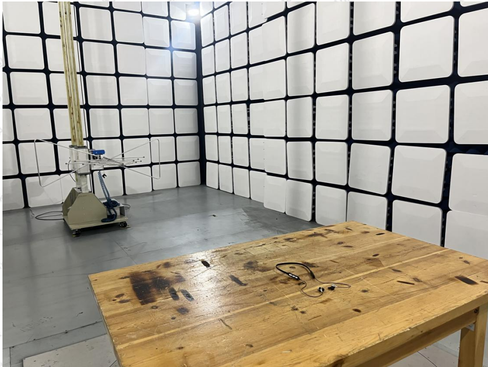
Photo of Radiation Emission Test
