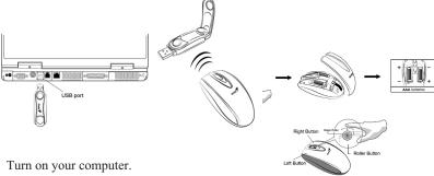
4. After you open Windows, please press the button on the receiver first and then press the button under the mouse for channel setting.
