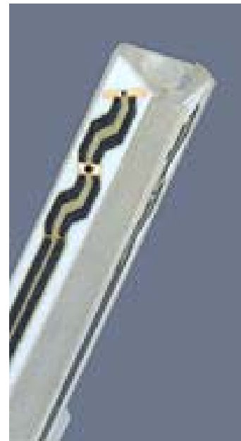
Inside view of ET3DV6 E-field Probe
