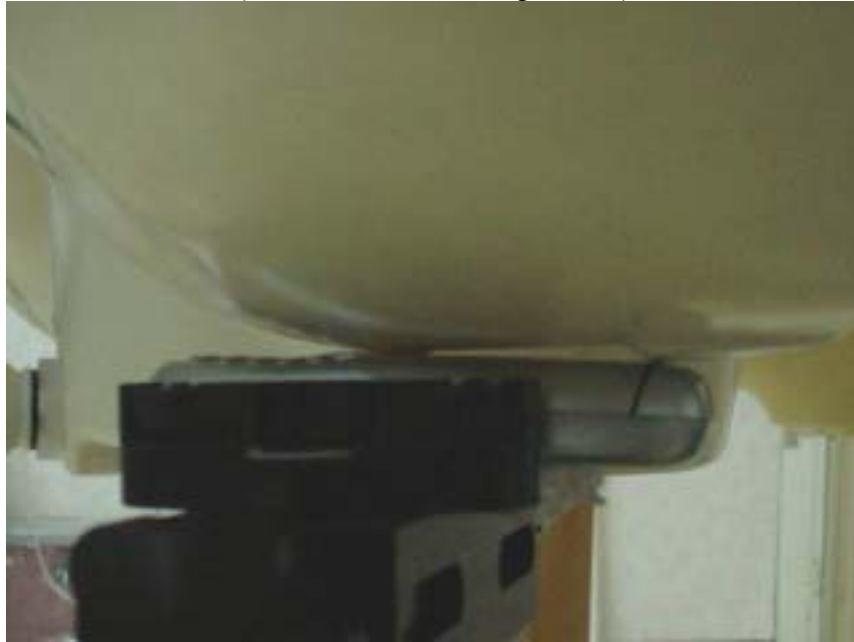
EUT Setup Configuration 2 (Left Head - Touched position)
