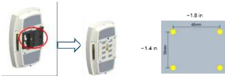
Figure 20: Mark Holes for Drilling
