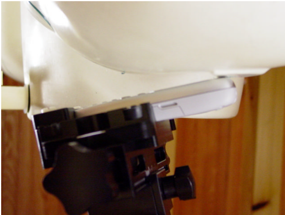
Figure 12.3 phone against the head (left tilt position)
