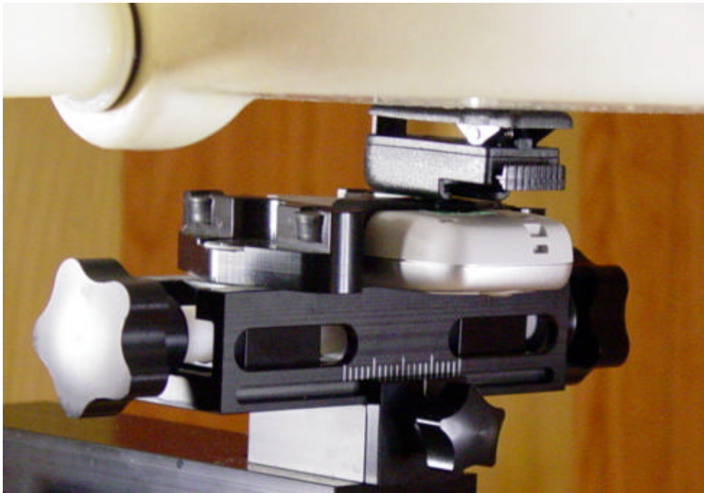
Figure 12.5 Body SAR Set-up (with phone clip)
