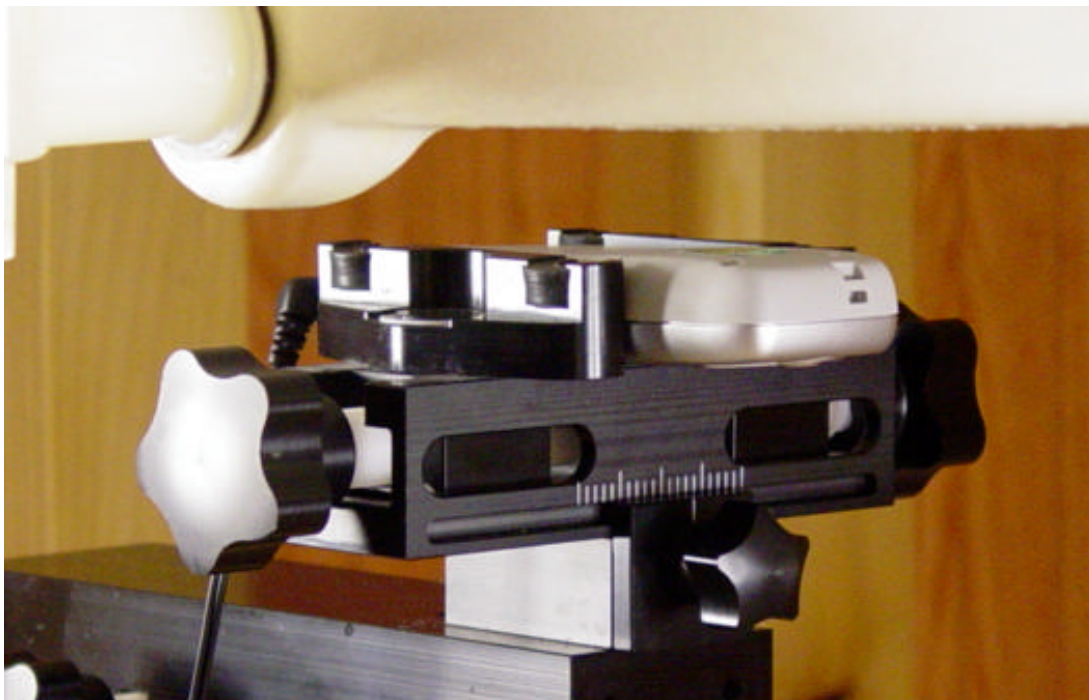
Figure 10.6 Body SAR Set-up (with 25mm air separation)
