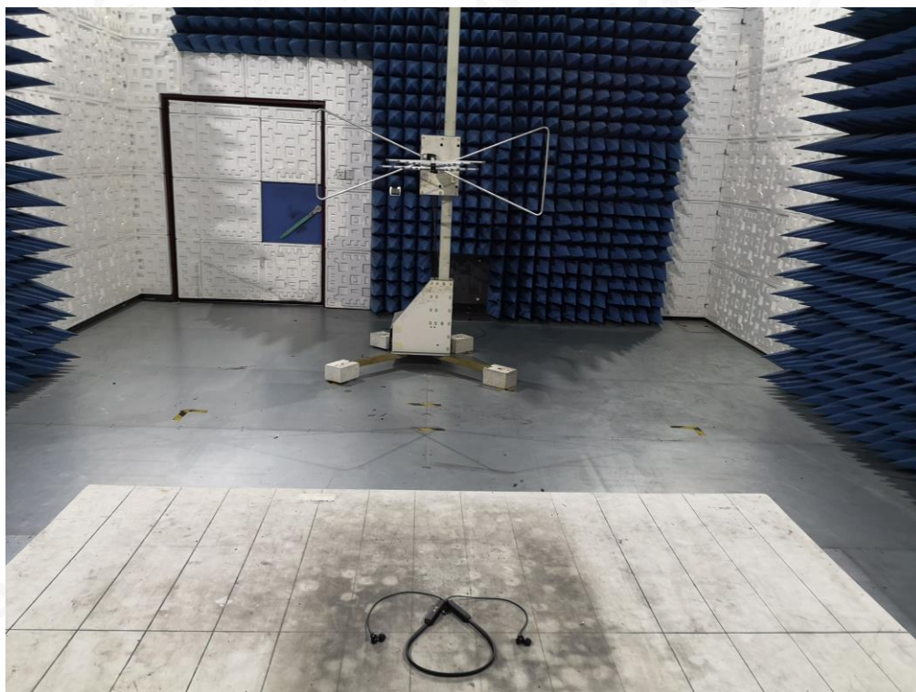
RADIATED EMISSION TEST SETUP ABOVE 1GHZ
