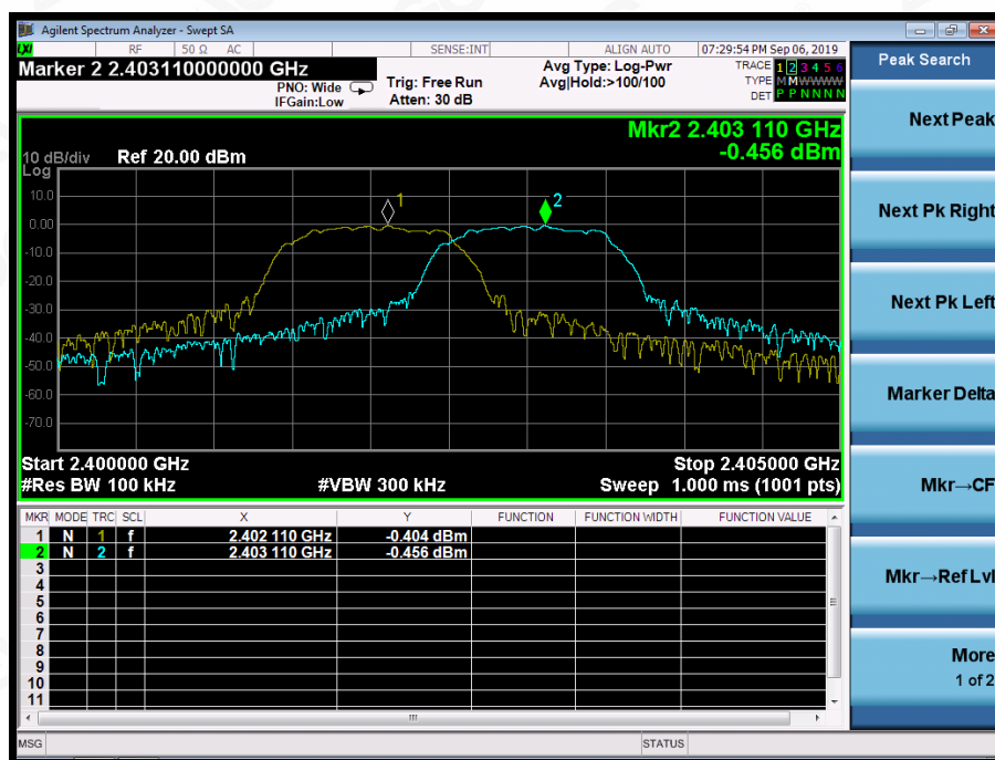
TEST PLOT FOR FREQUENCY SEPARATION
