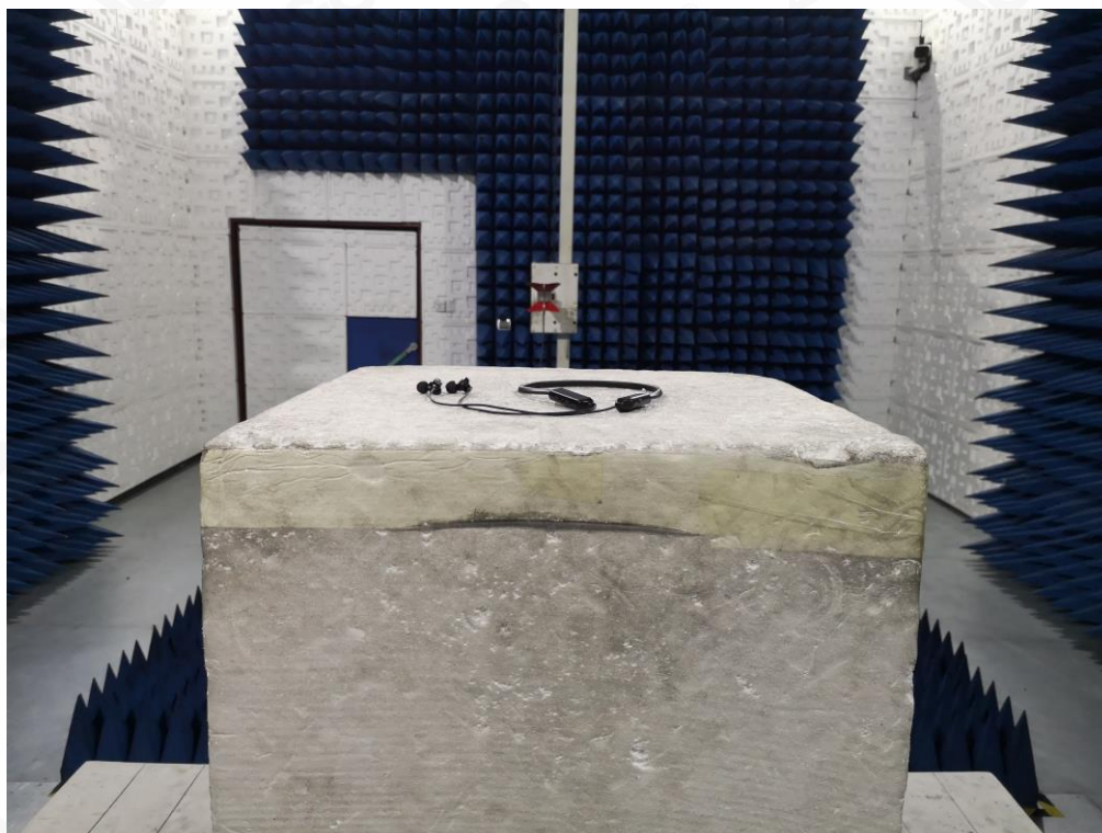
RADIATED EMISSION TEST SETUP ABOVE 1GHZ
