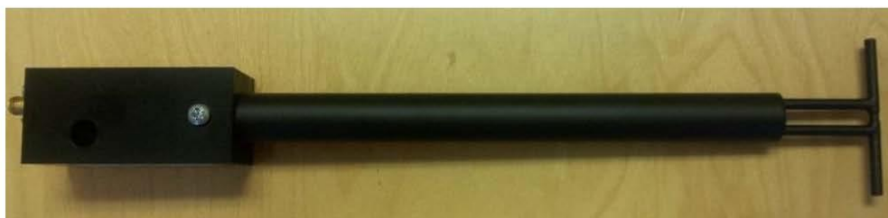
Figure 1 – MVG COMOSAR Validation Dipole
