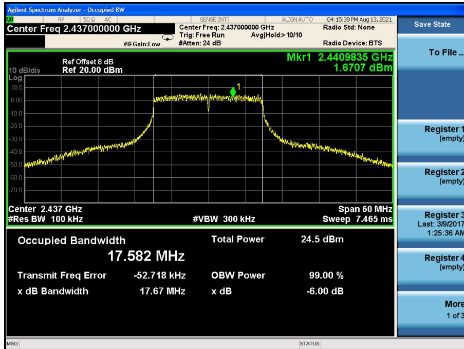
Fig.79 6dB Bandwidth: Ch6,11n
