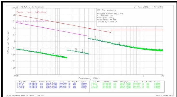
Note: The anechoic chamber has been properly calibrated so that the measurement results correspond to what would be obtained from an open field sites.
