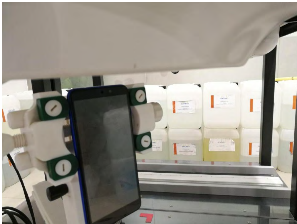
Top Edge(separation distance is 10mm)
