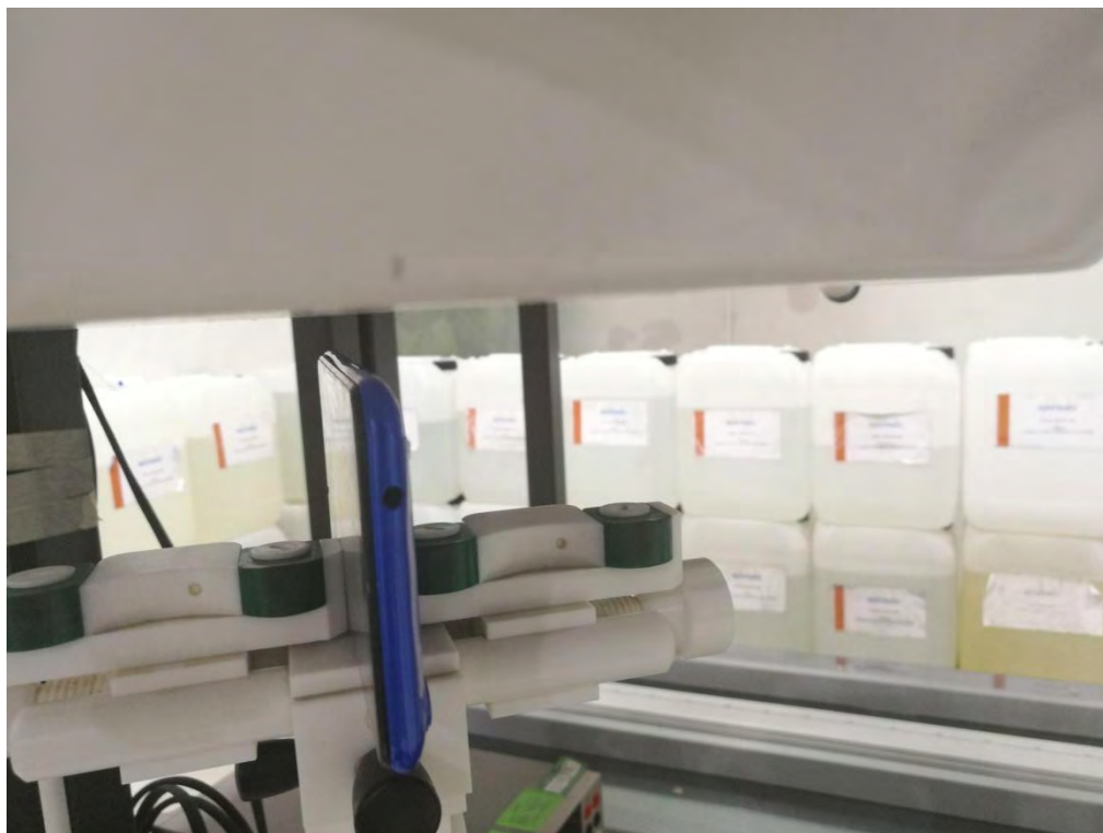
Left Edge(separation distance is 10mm)
