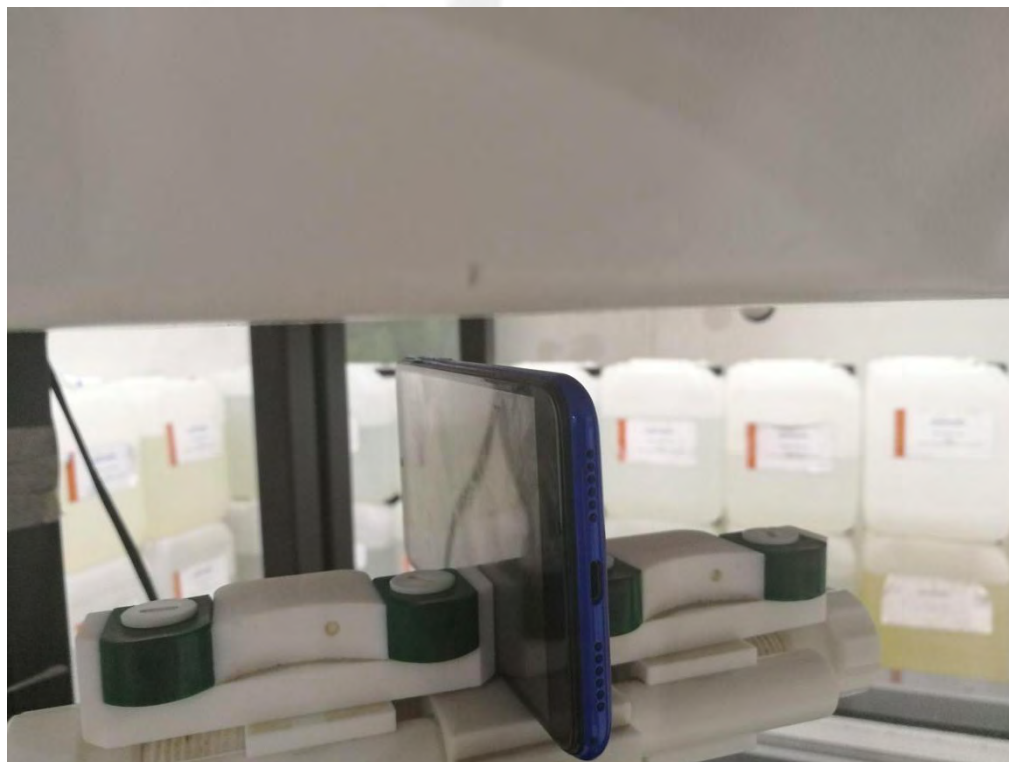
Right Edge(separation distance is 10mm)
