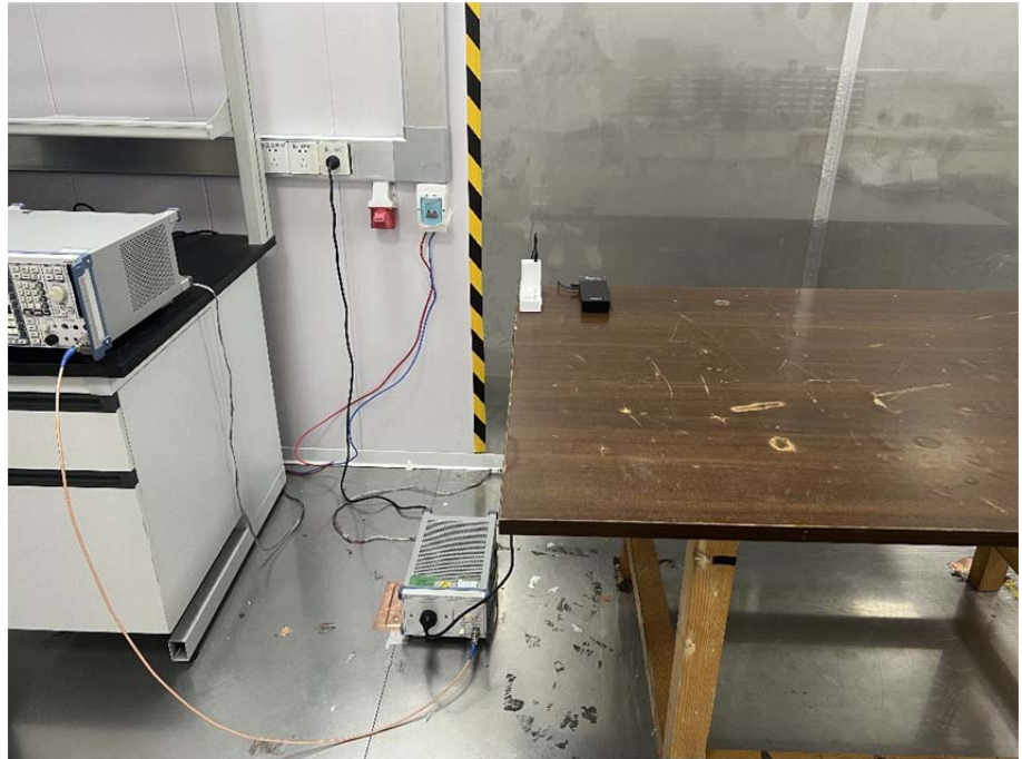
Conducted Emission Test Setup
