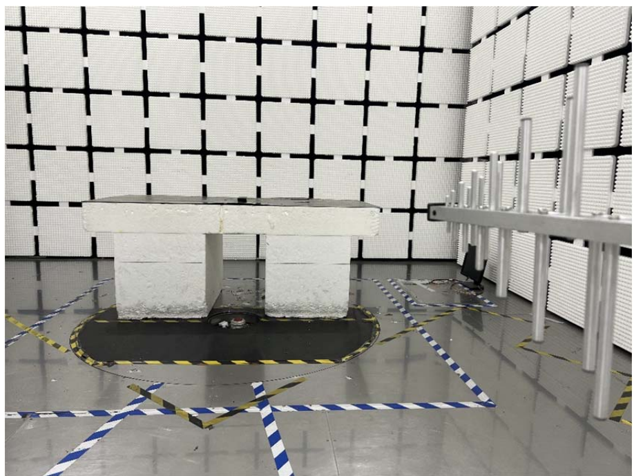
Radiation Emission Test Setup (30MHz to 1GHz)
