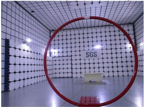
1.2 Radiated Emissions (30MHz-1GHz) Test Setup
