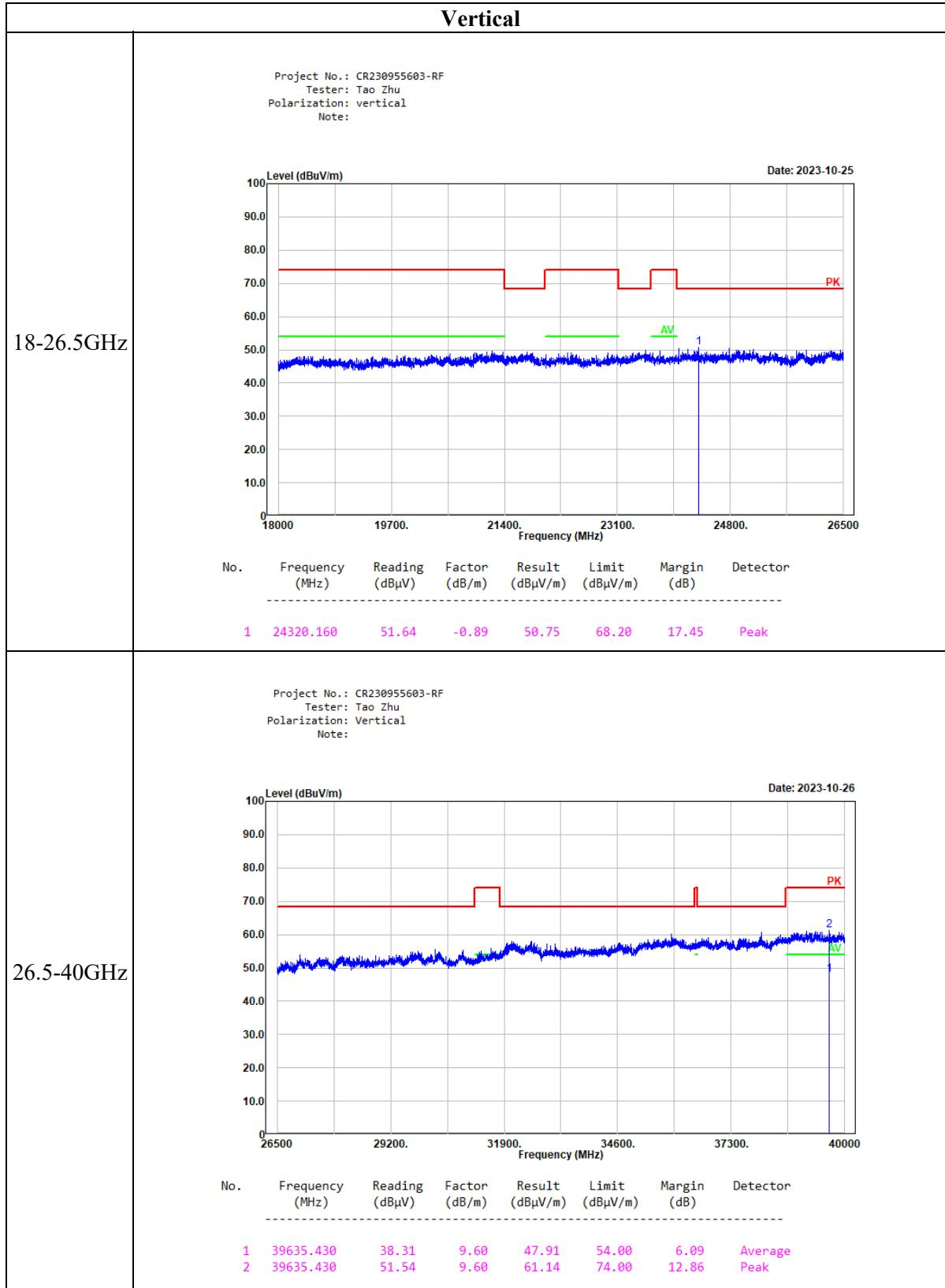
**Test plots for Band Edge Measurements (Radiated)****QPSK 1.4M**
