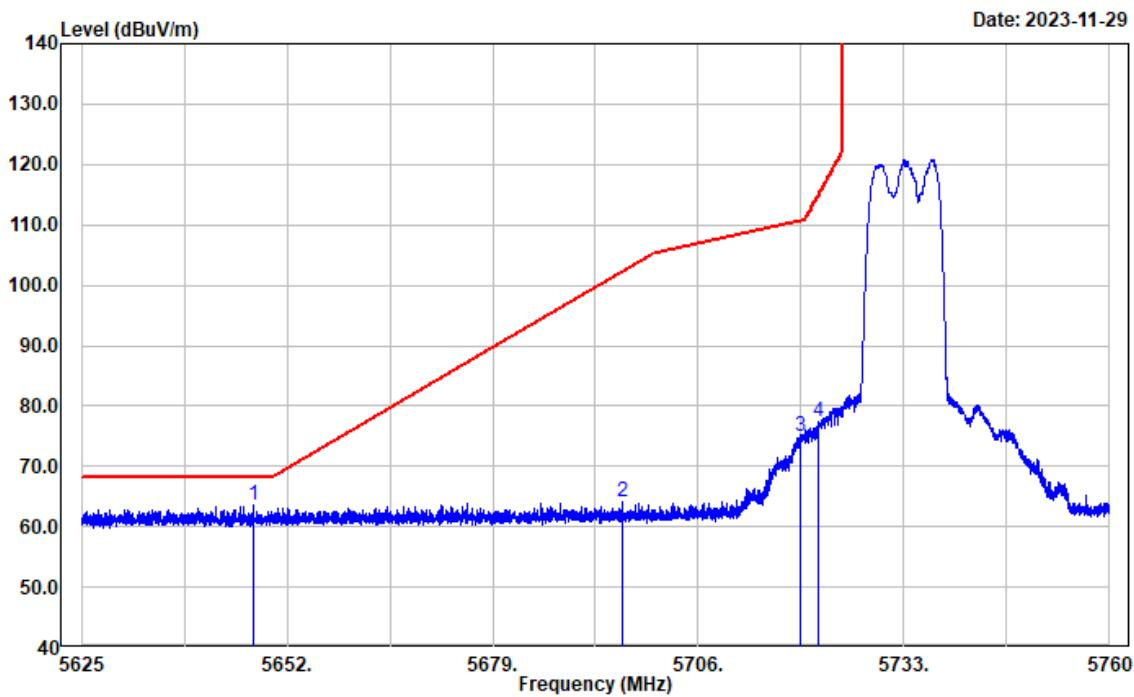
**16-QAM 10M****Test Channel: 5842MHz Ant. Polar. : Vertical**
