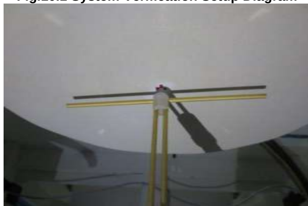
Fig.10.2 Photo of Dipole setup
